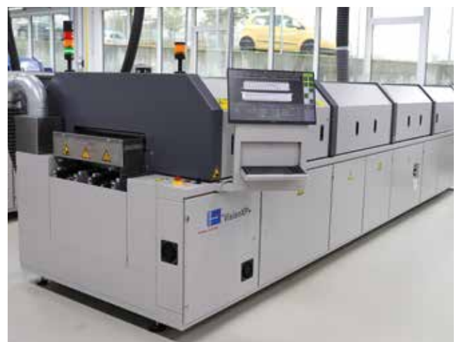
Patented mechatronic curtain, intake suction, ergonomic screen – resource-efficient redesign.
