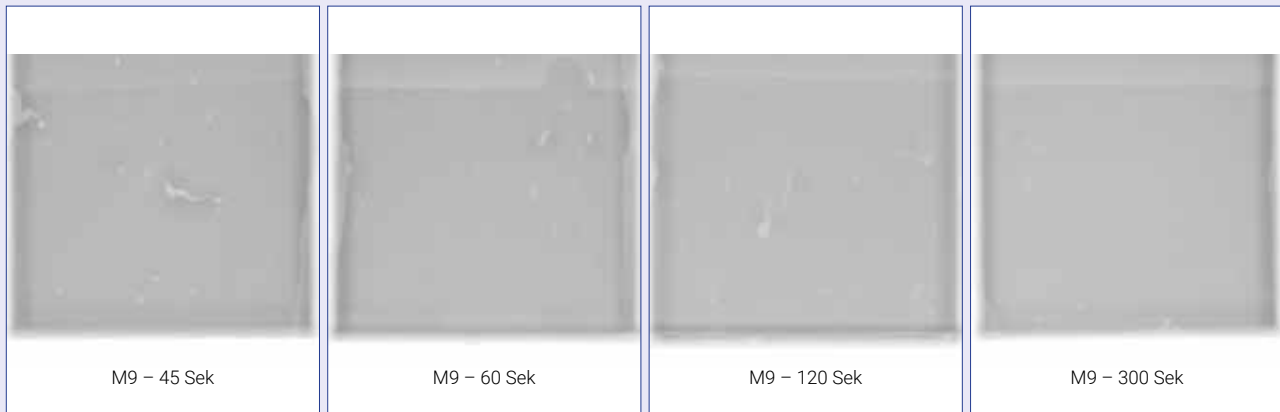
Figure 5 a-d: X-ray images of dummy solder joints for activation times ranging from 45 to 300 seconds.
