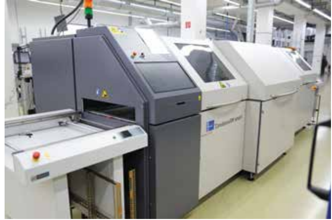
Hannusch also relies on Rehm systems for vapour phase soldering – in this case, the inline-capable CondensoxM Smart.
