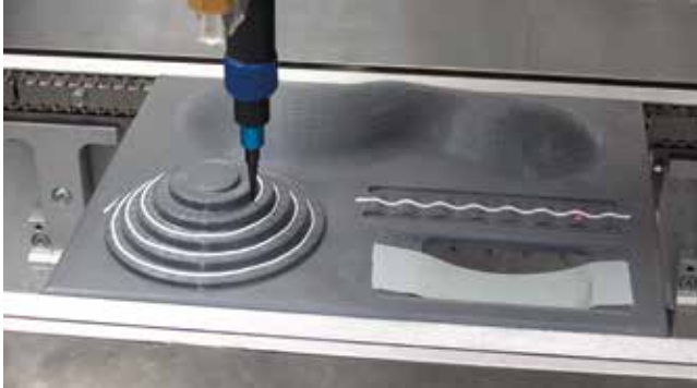
Precise material application on complex geometry
