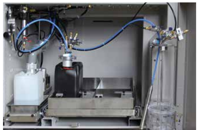
Easily accessible lacquer supply at the back of the plant
