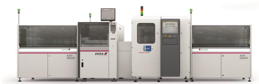
Figure 2: Example line with the R2R system from Rehm and Asys modules (Image: Asys)
