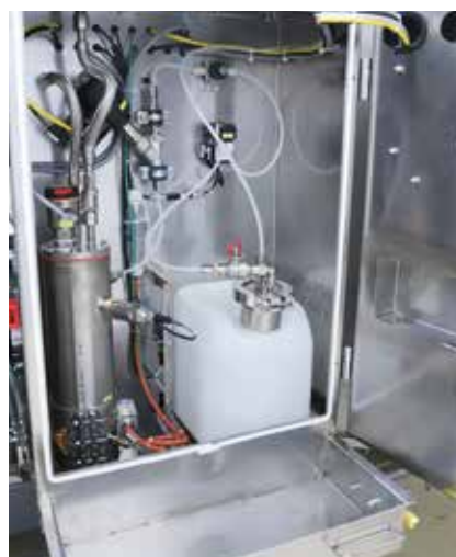
Extendable formic acid bubbler unit
