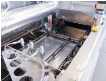
Goods carrier with flexible width setting to accommodate circuit boards with different transport widths
