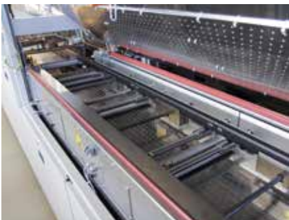
Segmented cooling tract with automatic width adjustment for each zone for the processing of different circuit board sizes
