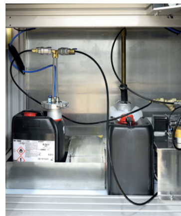
Lacquer supply at the front of the plant (XC) 前端涂料供应装置(XC)
