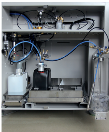
Easily accessible lacquer supply at the back of the plant (XP) 易于操作的后端涂料供应装置(XP)
